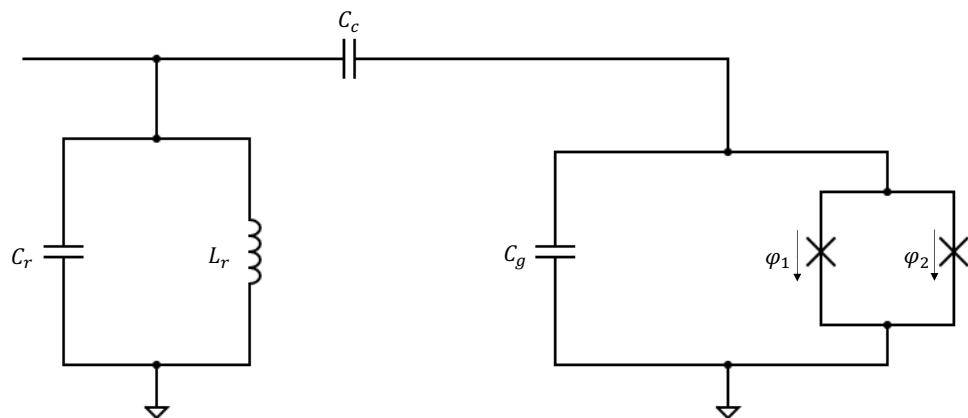
Figure 2: Circuit diagram of the SQUIDed transmon.
