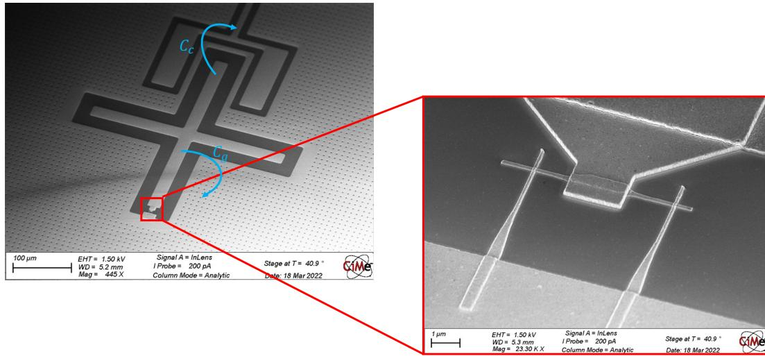
Figure 1: SEM pictures of a SQUIDed transmon (HQC) coupled to a readout resonator. The picture in the right is a zoom in of the picture on the left.
