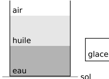
$$\rho_{\text{eau}} = 10^3 \text{ kg m}^{-3}, \rho_{\text{glace}} = 0.9 \cdot 10^3 \text{ kg m}^{-3}, \rho_{\text{huile}} = 0.85 \cdot 10^3 \text{ kg m}^{-3}, c_{\text{eau}} = 4 \cdot 10^3 \text{ J kg}^{-1} \text{ K}^{-1}, \\ c_{\text{glace}} = 2 \cdot 10^3 \text{ J kg}^{-1} \text{ K}^{-1}, c_{\text{huile}} = 1.8 \cdot 10^3 \text{ J kg}^{-1} \text{ K}^{-1}, \lambda_{\text{sol-liq,eau}} = 3.3 \cdot 10^5 \text{ J kg}^{-1}$$
