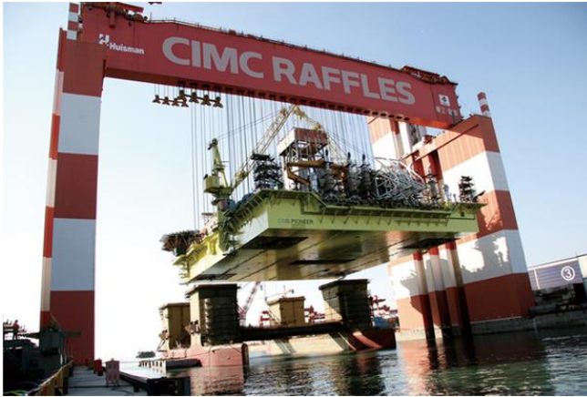
Taisun, Yantai, 2009 Lifting capacity 20 000 t Width 120 m Height 80 m
