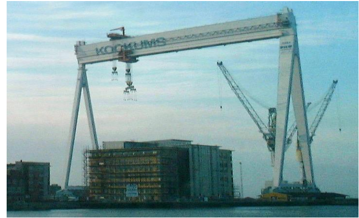
Kockums, Malmö 1974 Lifting capacity 1500 t Width 175 m Height 138 m
