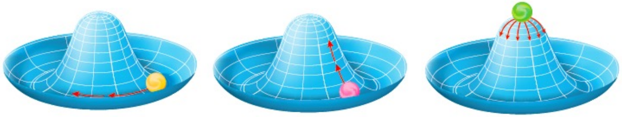
Figure 6.1: The “Mexican hat” potential. The masses of the two scalar DoF correspond to the second derivative of the potential around the minimum. One direction (left) is flat, while the other (center) is not. The plot on the right shows the symmetric maximum. It is unstable and does not correspond to a particle. In the case of a global symmetry, the flat direction corresponds to the massless Goldstone boson, while the non-flat direction corresponds to the massive DoF. In the case of a local symmetry, the flat direction corresponds to the longitudinal component of the vector boson, while the non-flat direction corresponds to the massive Higgs boson.
