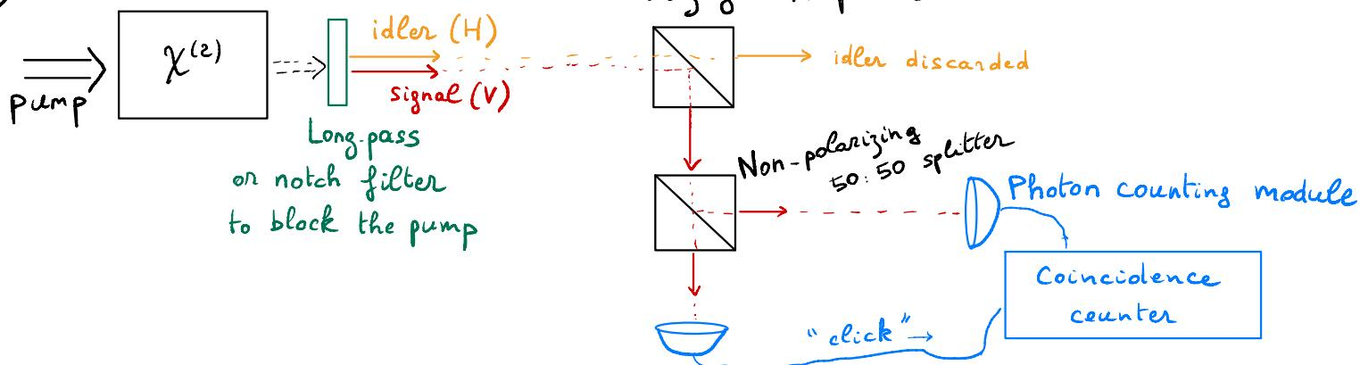
To a good approximation,  $g^{(2)}$  is given by the ratio of double-coincidence counts to the product of single counts on the two detectors. See this paper for full details:
