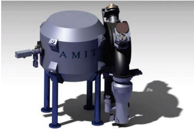
C. Oliver, CIEMAT, Spain et al. superconducting cyclotron, B=4 Tesla
