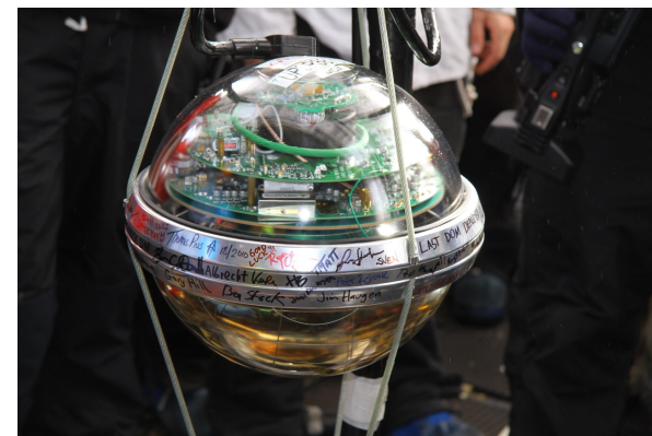
DOM (digital optical module) PMT diameter: 10 inches
