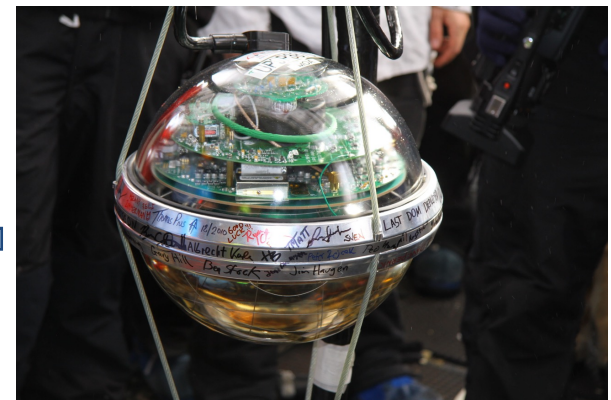
DOM (digital optical module) PMT diameter: 10 inches
