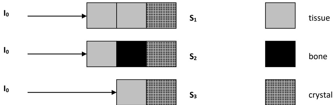
The intensity of signal (light) produced by the crystal is proportional to the attenuation of X-rays within the crystal.
