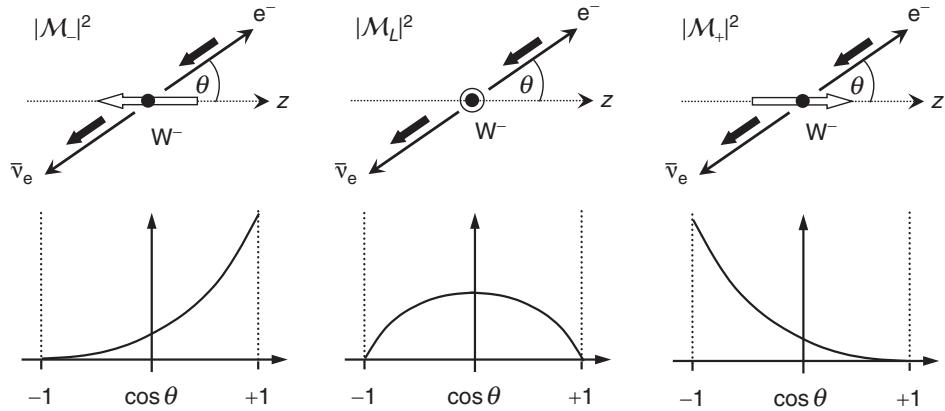
**Fig. 15.3** The angular distributions of the electron and electron antineutrino in the decay  $W^- \rightarrow e^- \bar{\nu}_e$  for the three possible W-boson polarisation states.
