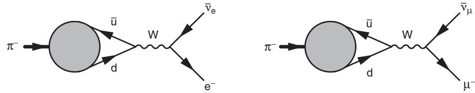
**Fig. 11.7** Two of the three main decay modes for the  $\pi^-$ . The decay  $\pi^- \rightarrow \mu^- \bar{\nu}_\mu \gamma$  (not shown) has a comparable branching ratio to that for  $\pi^- \rightarrow e^- \bar{\nu}_e$ .
