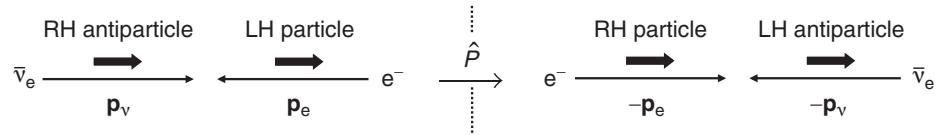
Fig. 11.5 The allowed helicity combination for a  $e^- \bar{\nu}_e$  weak interaction, and (right) its parity transformed equivalent.
