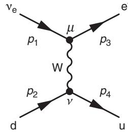
Fig. 11.3 The lowest-order Feynman diagram for the charged-current weak interaction  $\nu_e d \rightarrow e^- u$ .
