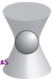
bead pulled to center of an optical trap
