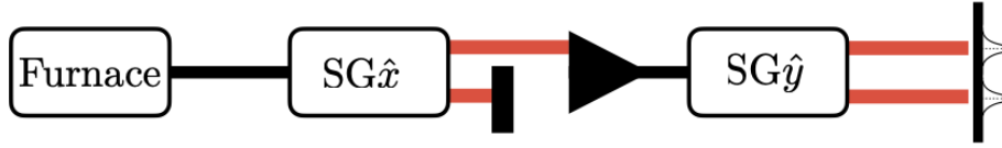
Figure 2.2: Experiment with two SG devices aligned in the x and y directions, respectively and blocking one component before entering the second device. All atoms emerge with the unfiltered state. Notice that in this case atoms exiting the furnace arrive from the z direction.
