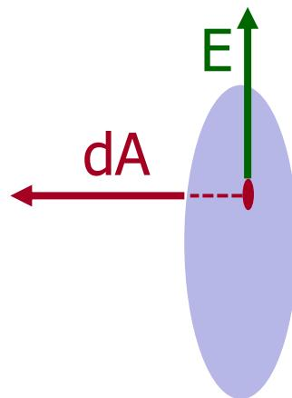
$$\vec{E} \cdot d\vec{A} = 0 \text{ because } \vec{E} \perp d\vec{A}$$
