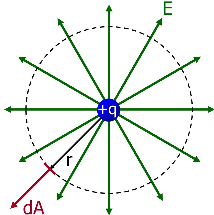
The direction of  $\vec{E}$  is shown in the diagram.
