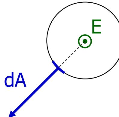
The angle between  $\vec{E}$  and  $d\vec{A}$  is  $90^\circ$ .
