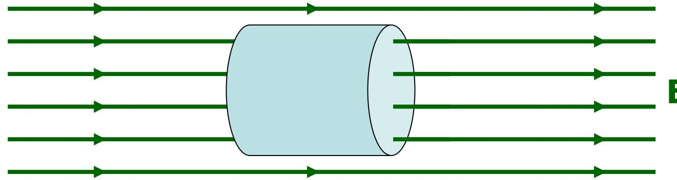
Electric Flux Example: Calculate the electric flux through a cylinder with its axis parallel to the electric field direction.
