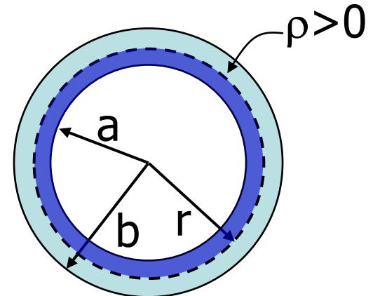
$$q_{\text{enclosed}} = q_{\text{shell of inner radius } a \text{ and outer radius } r}$$
