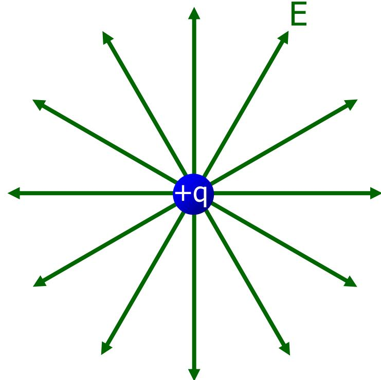
Example: use Gauss' Law to calculate the electric field from an isolated point charge  $q$ .
