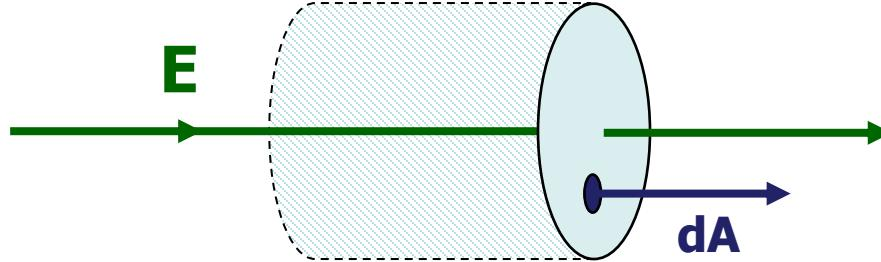
Every  $d\vec{A}$  on the right end cap is parallel to  $\vec{E}$ . The angle between the two vectors is  $0^\circ$
