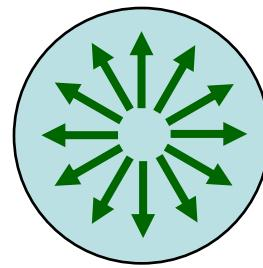
Inside the charged cylinder, by symmetry  $\vec{E}$  must be radial.
