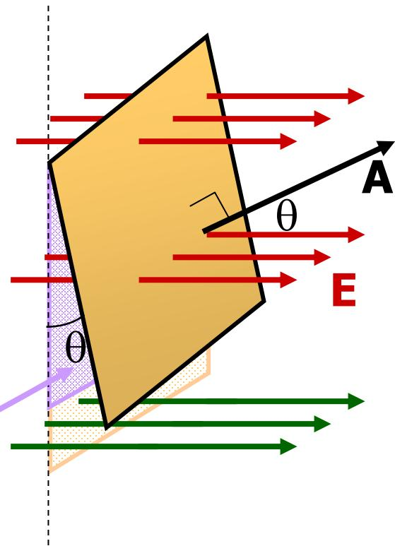
Therefore, the amount of surface area effectively “cut through” by the electric field is  $A \cos \theta$ .
