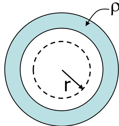
Answer: Pick any charge on the shell. Assume a positive charge so you can draw an electric field line. Draw an electric field line from the charge out to infinity. The line never goes into the sphere (and if it did, it would go out anyway, because there is no - charge to “land on”). It contributes nothing to the flux.
