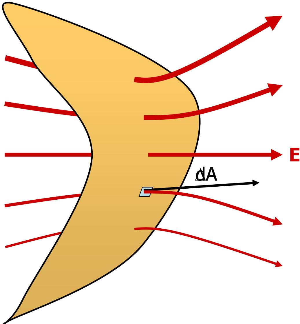
divide the surface into infinitesimal surface elements and add the flux through each...
