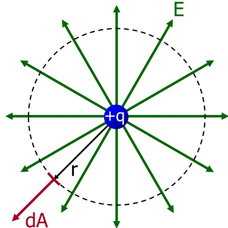
Everywhere on the sphere,  $\vec{E}$  and  $d\vec{A}$  are parallel and  $E$  is constant so
