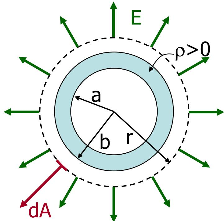
**Summary:** electric field for  $0 < r < \infty$  for an insulating spherical shell of inner radius  $a$ , outer radius  $b$ , and with a uniform volume charge density  $\rho$  spread throughout shell.
