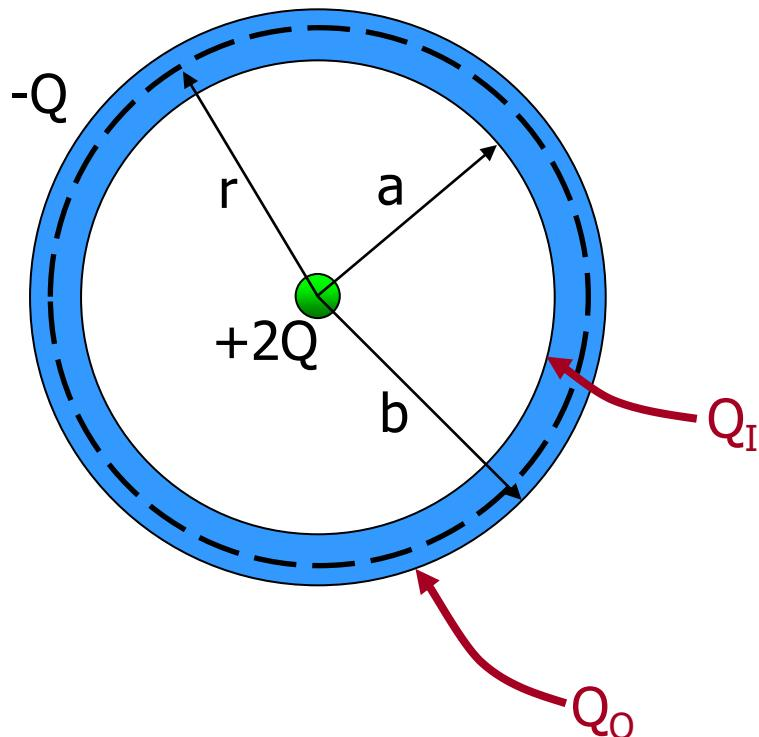
From Gauss' Law we know that excess\* charge on a conductor lies on surfaces.
