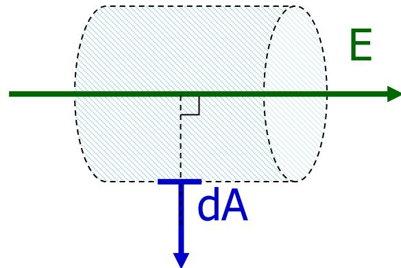
$$\int_{tube} \vec{E} \cdot d\vec{A}_{tube} = \int_{tube} E dA_{tube} \cos 90^\circ = \int_{tube} 0 dA_{tube} = 0$$
