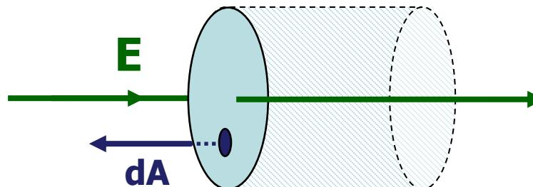
Electric Flux Example: Calculate the electric flux through a cylinder with its axis parallel to the electric field direction.
