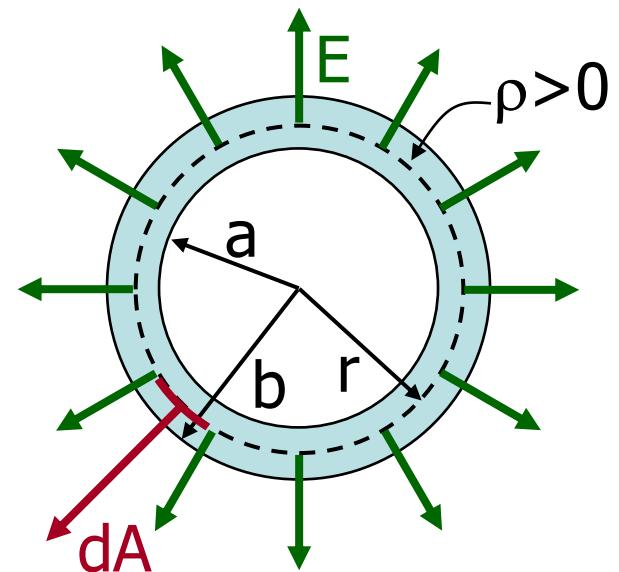
The hard part is finding  $q_{\text{enclosed}}$ . We have to determine the charge inside the dashed-line Gaussian sphere.
