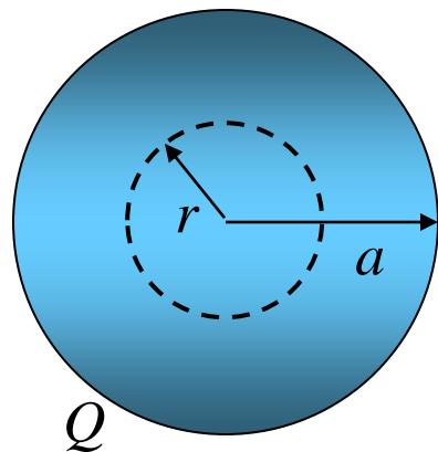
$$\oint \vec{E} \cdot d\vec{A} = \frac{q_{\text{enclosed}}}{\epsilon_0} = \frac{\rho V_{\text{enclosed}}}{\epsilon_0}$$
