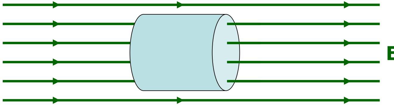
The net electric flux through a closed cylindrical surface is zero.
