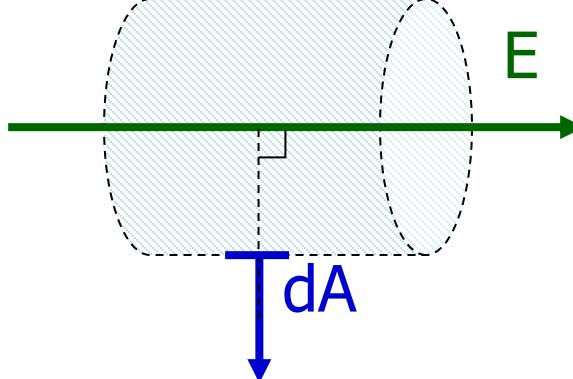
The angle between  $\vec{E}$  and  $d\vec{A}$  is  $90^\circ$ .
