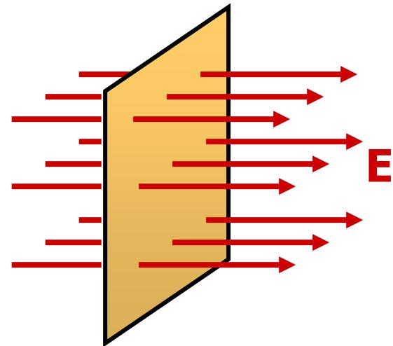
The **electric flux** passing through a surface is the number of electric field lines that pass through it.
