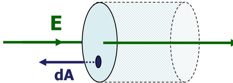
Every  $d\vec{A}$  on the left end cap is antiparallel to  $\vec{E}$ . The angle between the two vectors is  $180^\circ$
