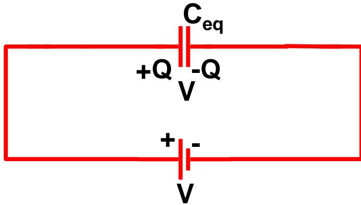
“equivalent” means it has the same charge  $Q$  and the same voltage drop  $V$  as the three capacitors
