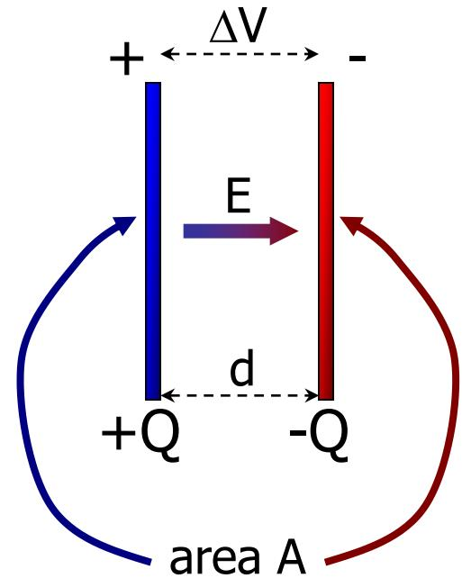
The “volume of the capacitor” is  $\text{Volume} = Ad$
