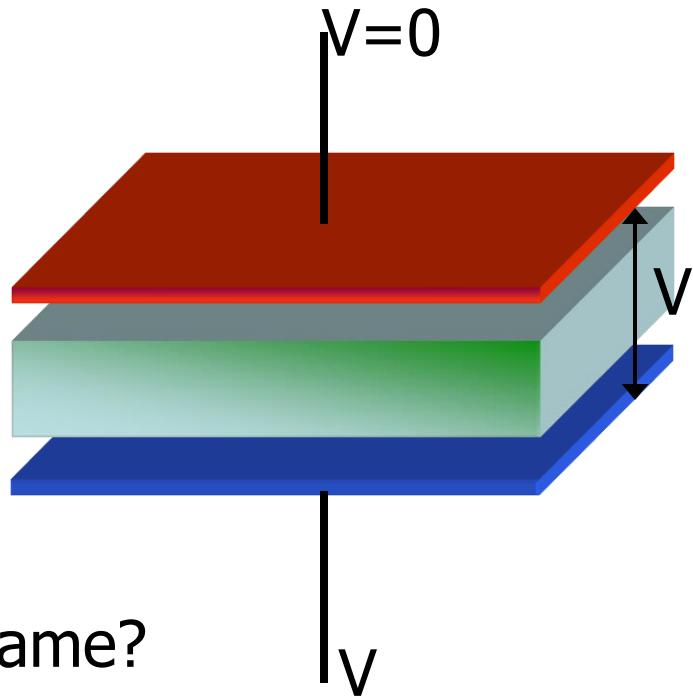
Example: a parallel plate capacitor has an area of  $10 \text{ cm}^2$  and plate separation 5 mm. A 300 V battery is connected to its plates. If neoprene is inserted between its plates, how much charge does the capacitor hold.
