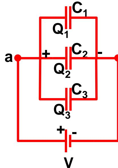
Imagine replacing the parallel combination of capacitors by a single **equivalent capacitor**
