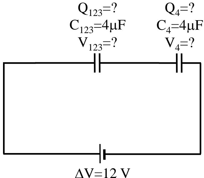
C<sub>4</sub> is in series with C<sub>123</sub> and together they form C<sub>eq</sub>.
