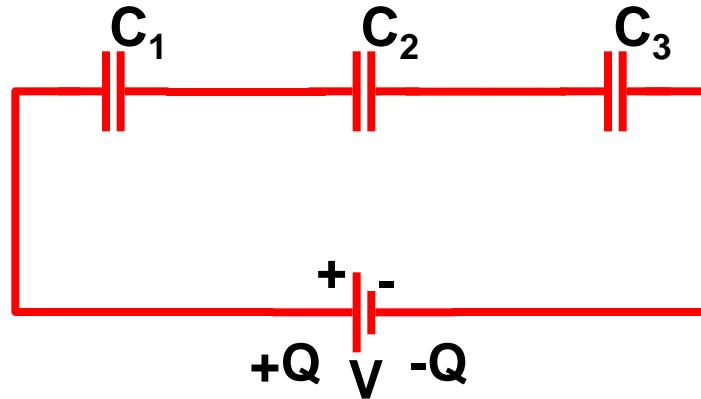
charge  $+Q$  flows from the battery to the left plate of  $C_1$
