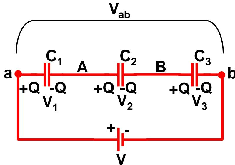
The charges on  $C_1$ ,  $C_2$ , and  $C_3$  are the same, and are
