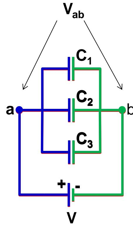
all three capacitors must have the same potential difference (voltage drop)  $V_{ab} = V$
