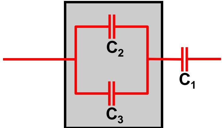
Start by combining parallel combination of  $C_2$  and  $C_3$
