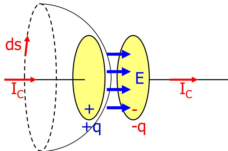
$\kappa$  Is the dielectric constant of the medium in between the capacitor plates. In the diagram, with an air-filled capacitor,  $\kappa = 1$ .
