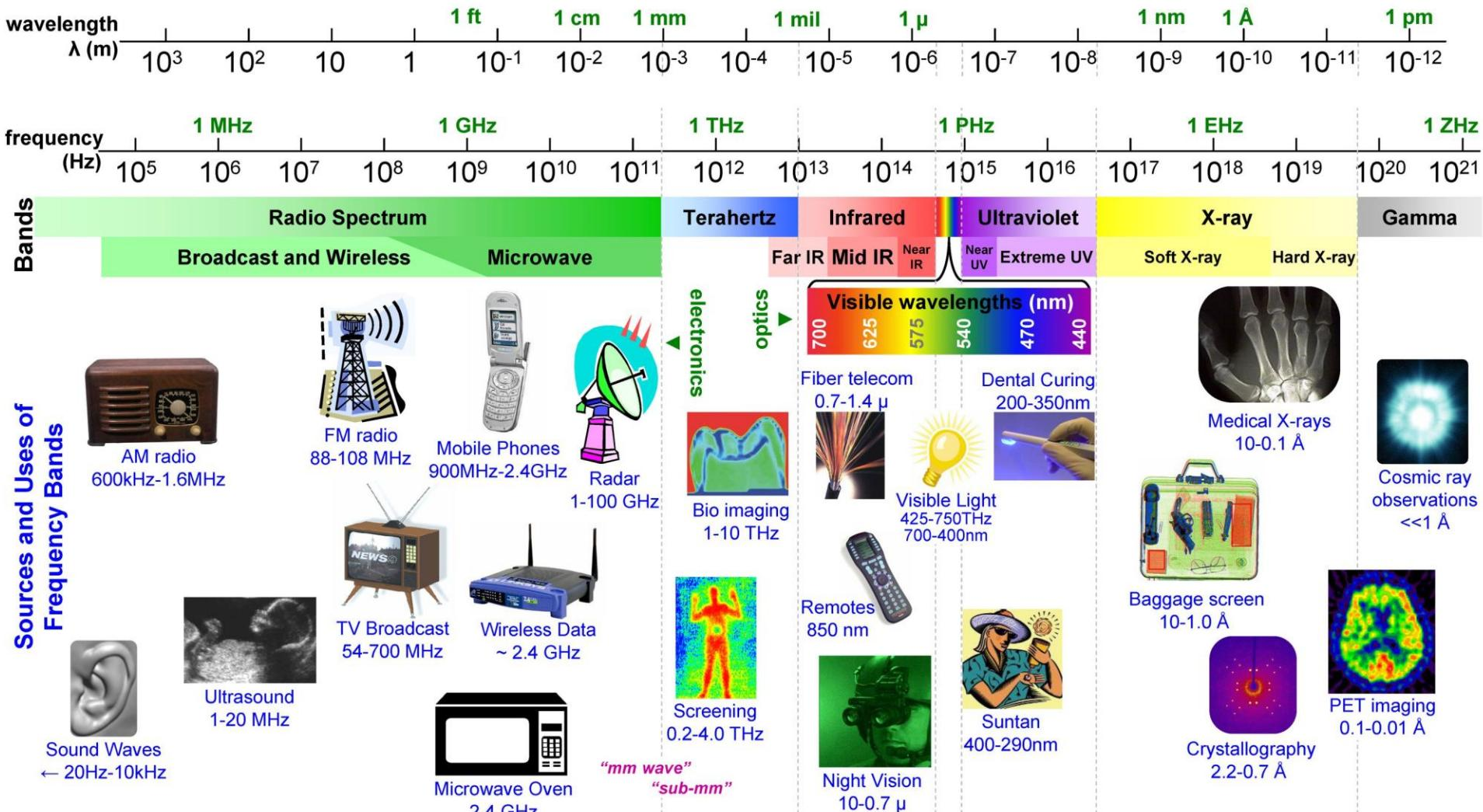
$$\lambda = 3 \times 10^8 / \text{freq} = 1 / (\text{wn} \times 100) = 1.24 \times 10^{-6} / \text{eV}$$
