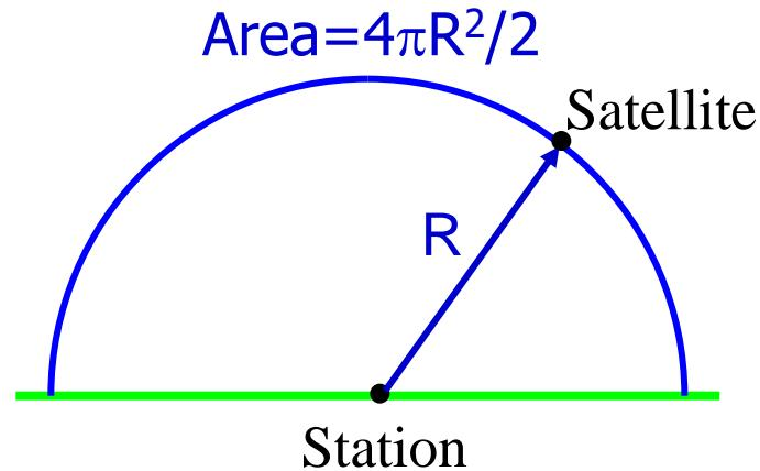
$$I = \left( \frac{\text{power}}{\text{area}} \right)_{\text{average}} = \frac{P}{2\pi R^2} = \frac{(5.00 \times 10^4 \text{ W})}{2\pi (1.00 \times 10^5 \text{ m})^2} = 7.96 \times 10^{-7} \text{ W/m}^2$$
