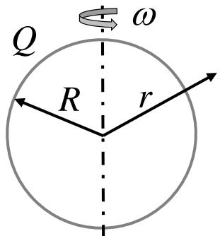
$$ds = Rd\theta R \sin \theta d\varphi = R^2 \sin \theta d\theta d\varphi \quad dq = \sigma ds \quad \sigma = Q / 4\pi R^2$$
