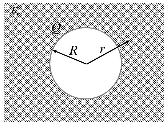
$$\text{Sym. sphérique + Gauss: } \int_S \mathbf{D} \cdot d\mathbf{s} = \int_V \rho_f dV \Rightarrow D 4\pi r^2 = \begin{cases} 0 & \text{pour } r < R \\ Q & \text{pour } r < R \end{cases} \Rightarrow D = \begin{cases} 0 & \text{pour } r < R \\ \frac{1}{4\pi} \frac{Q}{r^2} & \text{pour } r < R \end{cases}$$
