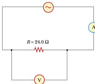
**Solution:** The meters measure the rms values of potential difference and current. These are  $V_{\text{rms}} = \frac{V_0}{\sqrt{2}} = 70.7$  V and  $I_{\text{rms}} = \frac{V_{\text{rms}}}{R} = 2.95$  A.  $\square$
