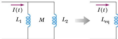
**Solution:** With  $I = I_1 + I_2$ , the voltage across the pair is:  $\Delta V = -L_1 \frac{dI_1}{dt} - M \frac{dI_2}{dt} = -L_2 \frac{dI_2}{dt} - M \frac{dI_1}{dt} = -L_{\text{eq}} \frac{dI}{dt}$ . Hence,  $-\frac{dI_1}{dt} = \frac{\Delta V}{L_1} + \frac{M}{L_1} \frac{dI_2}{dt}$  and  $-L_2 \frac{dI_2}{dt} + \frac{M \Delta V}{L_1} + \frac{M^2}{L_1} \frac{dI_2}{dt} = \Delta V$ , yielding
