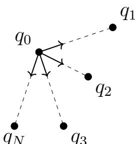
$$\vec{F}_{q_1, q_2, \dots, q_N \rightarrow q_0} = \sum_{j=1}^N \frac{1}{4\pi\epsilon_0} \frac{q_j q_0}{r_{q_j \rightarrow q_0}^2} \hat{r}_{q_j \rightarrow q_0} \quad (1.8)$$
