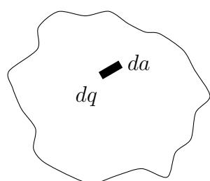
$$dq = \sigma da; \quad \sigma = \frac{dq}{da} \quad (1.11)$$
