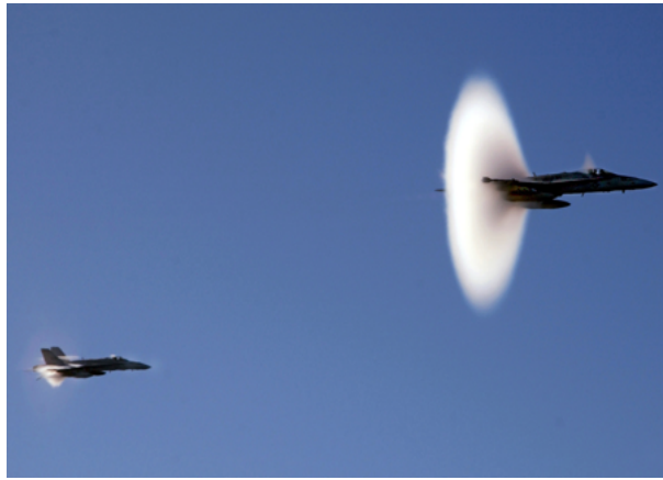
FIGURE 3.7 – L'onde de choc derrière un FA18 Hornet supersonique. (Source : http://wallpapers.windowsace.com/pics/-/1/-18-hornet-jet-planes-sonic-boom-supersonic-desktop-2100x1500-wallpaper-d-a-ibackgroundz.co )
