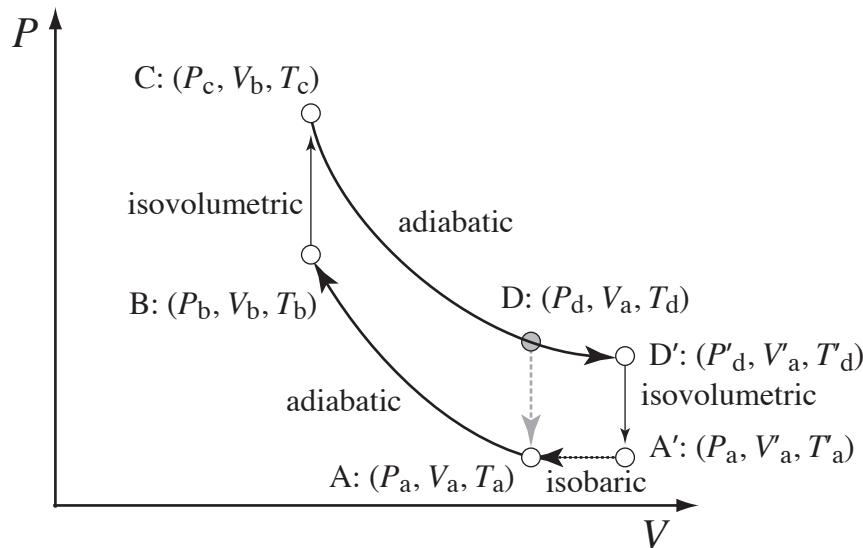
Show that an engine with Miller cycle ( $A \rightarrow B \rightarrow C \rightarrow D' \rightarrow A' \rightarrow A$ ) is more efficient than that with Otto cycle ( $A \rightarrow B \rightarrow C \rightarrow D \rightarrow A$ ).
