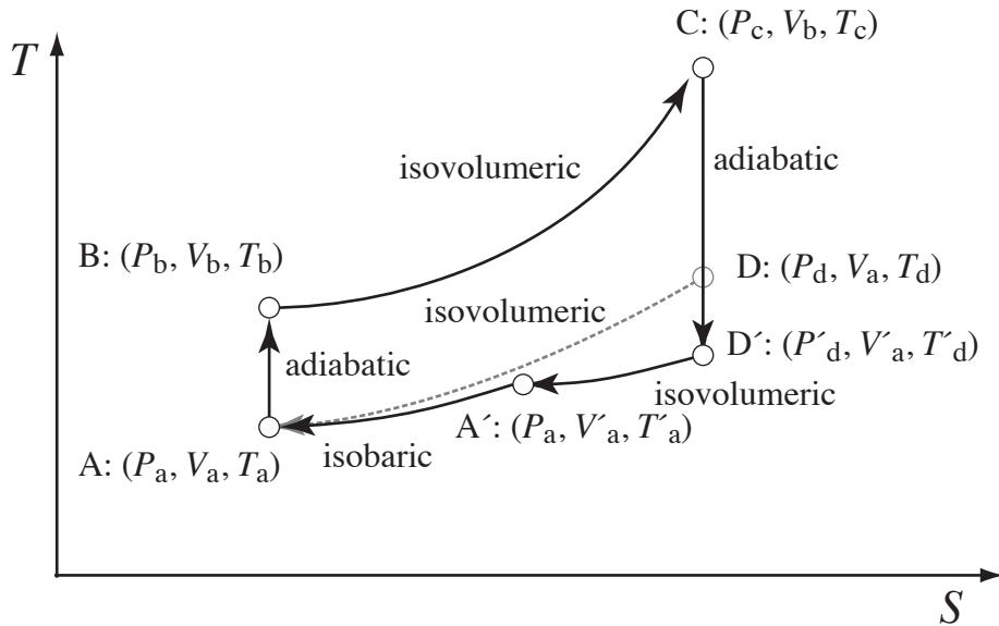
The thermal energy flow into the engine,  $Q_{\text{in}}$ , is the positive heat in the system given by the area below the  $B \rightarrow C$  line for both Otto and Miller cycles, thus  $Q_{\text{in}}^{\text{Otto}} = Q_{\text{in}}^{\text{Miller}}$ .
