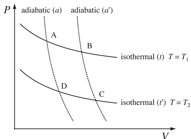
Volumes and pressures of the four crossing points, A, B, C and D are given by  $V_a, V_b, V_c, V_d$  and  $P_a, P_b, P_c, P_d$ , respectively. Along the isothermal line,  $t$ , we
