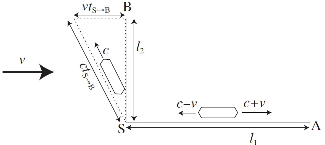
An example of a boat travels from the starting point S to and back with a velocity,  $c$ , to a destination A (distance S-A,  $l_1$ ) that is along the direction of the stream, and B perpendicular to the direction of the stream (distance S-B,  $l_2$ ). The velocity of the stream is  $v$ .
