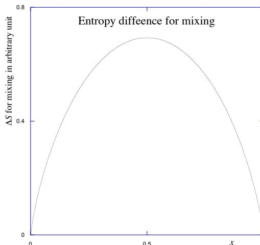
As seen from the figure above,  $\Delta S \geq 0$ , where  $\Delta S = 0$  at  $x = 0$  and  $= 1$ , i.e. with one gas and no mixing, and maximum at  $x = 0.5$ , i.e. mixing of two equal amount of gasses. This makes sense for two different ideal gasses. Since mixing two different gasses is an irreversible process.
