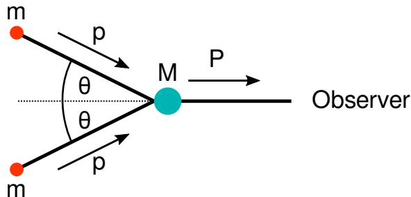
Two particles of known rest mass  $m$  are going with known total momentum  $p$  toward each other at a known angle  $\theta$  as indicated in the diagram. They collide and form a particle of unknown rest mass  $M$ , which moves in the direction as indicated with unknown momentum  $P$ . For simplicity, assume that we work in units such that  $c = 1$ .
