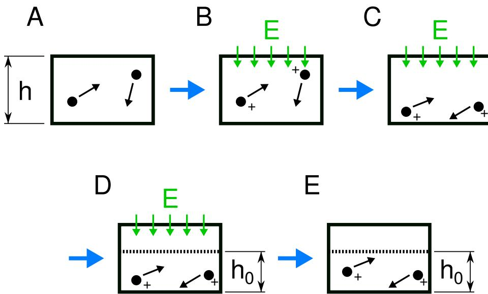
In this experiment, a monatomic gas of  $N$  atoms of mass  $m$  and charge  $q$  is in a thermally isolated box of volume  $V$  and height  $h$ . The following steps take place successively:
