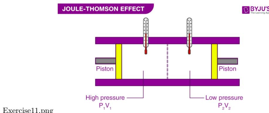
a) Show that the enthalpy  $H$  is conserved if the external pressures exerted by the pistons are equal to the pressures in the corresponding subsystems at all times, i.e.  $P_{1,ext} = P_1$  and  $P_{2,ext} = P_2$ . This is called the Joule Thomson expansion.
