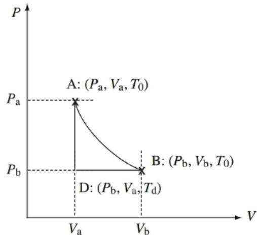
3) Work as a process-dependent Quantity: three processes are performed on a gas from a state given by  $P_1, V_1$  to a state given
