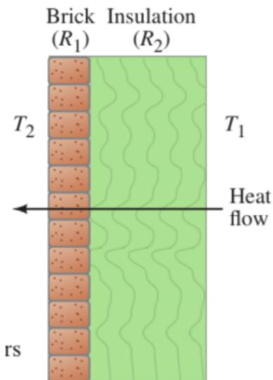
Definition of R values: the R value, i.e. the thermal resistance, specifies insulation properties of a building material, defined for a given thickness  $l$  of the material:  $R = l/k$  with  $k$  being the thermal conductivity.
