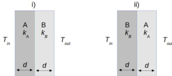
II) A pipe consists of the two layers of material with a same thickness  $d$ . The inner radius of the pipe is  $r_{in}$ . Two material A and B with thermal conductivities,  $k_A$  and  $k_B$ , respectively, are available for the layers where  $k_A > k_B$ . This pipe is used to transport hot water with a temperature  $T_{in}$  through cold outside with a temperature of  $T_{out}$ , where  $T_{in} > T_{out}$ . Figures below show the cross-sections of the pipes.
