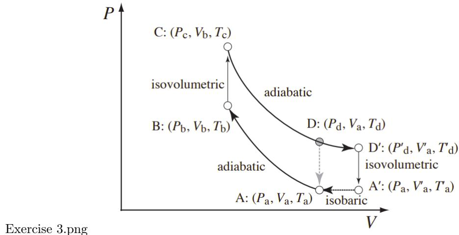
Show that an engine with Miller cycle ( $A \rightarrow B \rightarrow C \rightarrow D' \rightarrow A' \rightarrow A$ ) is more efficient than that with Otto cycle ( $A \rightarrow B \rightarrow C \rightarrow D \rightarrow A$ ).
