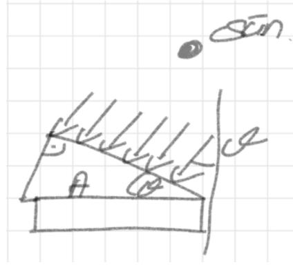
$\theta$  is the angle between sun rays and the line perpendicular to the area  $A \rightarrow A \cos(\theta)$  is the effective area at right angle to sun rays.
