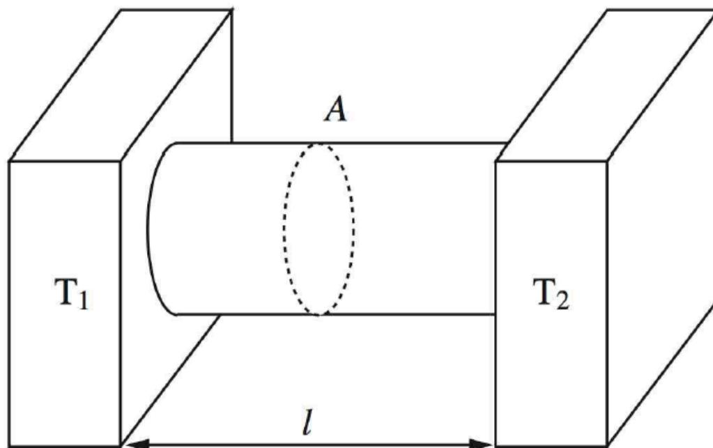
Heat bath 2 connected by a beam with  $Al$
