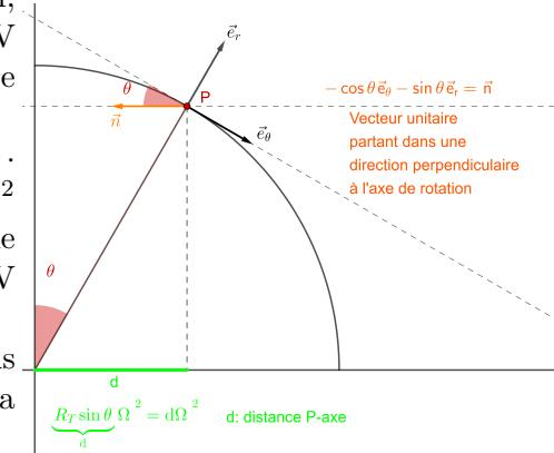
$$\begin{aligned} 2) 2\vec{\Omega} \wedge \vec{v}_{\mathcal{R}'}(P) \text{ (Coriolis)} \\ &= 2(\Omega \cos \theta \vec{e}_r - \Omega \sin \theta \vec{e}_\theta) \wedge v \vec{e}_\theta \\ &= 2\Omega v \cos \theta \vec{e}_r \wedge \vec{e}_\theta = 2\Omega v \cos \theta \vec{e}_\varphi \end{aligned}$$
