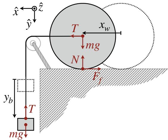
1. Consider the system composed of the wheel and the block (i.e. the two objects in the problem that move and have mass). Since we are asked about the state of the system at a particular *position* (i.e. after the center of the wheel has traveled a distance  $d$ ), it is best to use conservation of energy. If we were asked about the system after a given amount of time  $t$ , it would be easiest to use Newton's laws.
