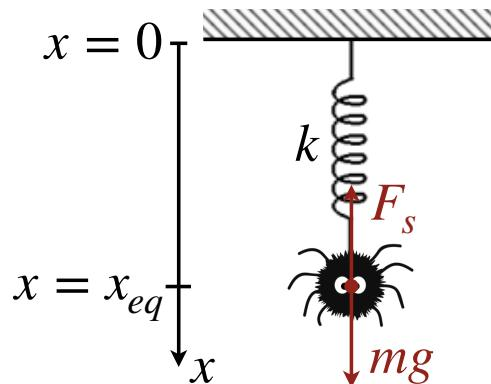
1. We will choose to use a one-dimensional Cartesian coordinate system with the origin defined to be the location of the ceiling. If the spider were located at  $x = 0$ , the spring would have a length of zero.
