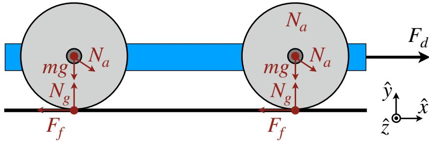
1. Due to the symmetry of the system, the free body diagram for all of the wheels is identical and is shown above. There are four forces on each wheel: gravity acting at the center of mass of the wheel (i.e. the center of the wheel), the normal force from the axle of the cart, the normal force from the ground, and the static friction force from the ground.
