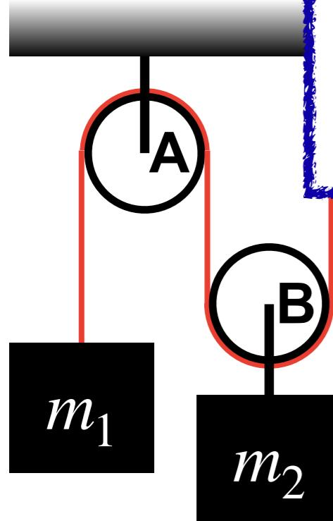
**A *constraint condition* is a requirement on the motion of objects due to the geometry of the system**
