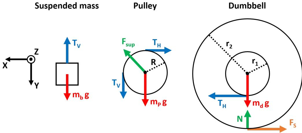
The "no slipping" condition suggests that static friction ( $F_s$ ) is acting on point  $C_2$ . This force acts in the negative x direction, opposing the tension force of the rope ( $T_H$ ).
