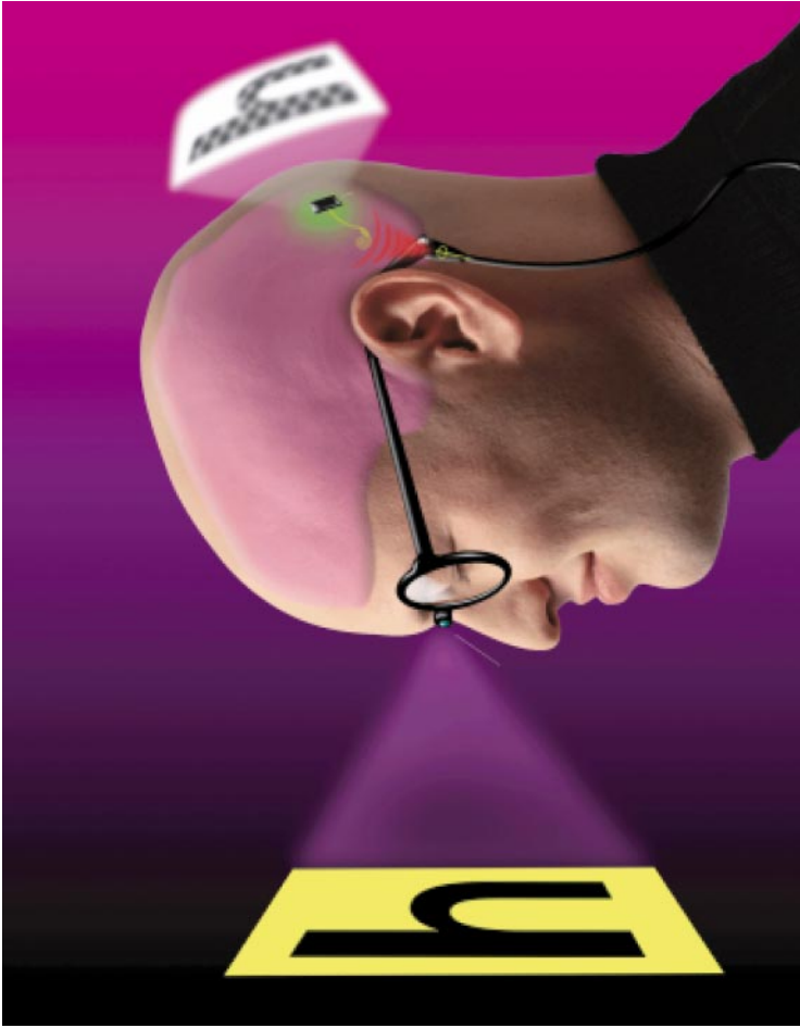
Figure 2 The components of a vision prosthesis must include a camera to convert light into electrical signals, a means of transforming visual space to the retinotopic organization of the target structure, a way to transmit power and control signals to implanted electronics, a way to stimulate multiple electrodes to generate the phosphenes, and an interface to the nervous system.
