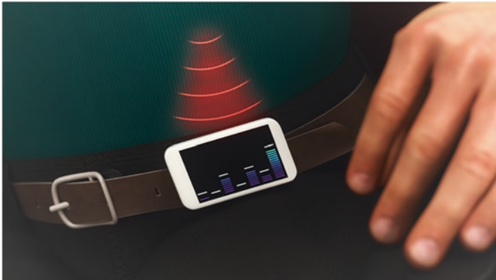
Fig. 7.20 Belt-worn processor receiving information from a wireless BCI and sending control patterns to an implanted wireless FES. (Courtesy of Wyss Center for Bio and Neuroengineering)
