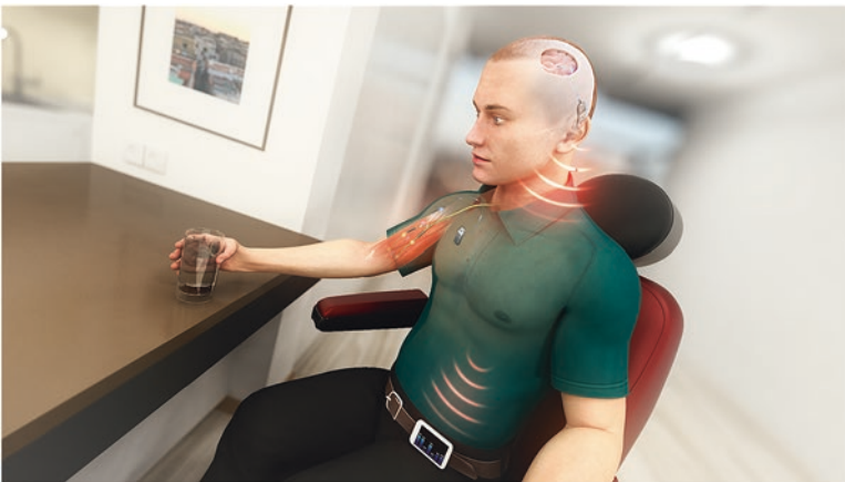
Fig. 7.22 Future vision of a fully implanted wireless system merging a FES activation of a paralyzed limb to a cortical sensing BCI with external wearable processor. (Courtesy of Wyss Center for Bio and Neuroengineering)
