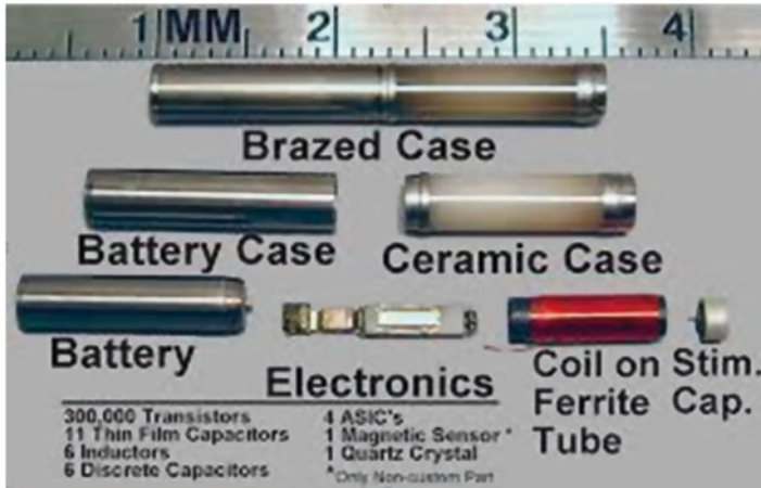
Fig. 4.25 Cylindrical brazen ceramic-Ti hermetic encapsulation, including battery, Bion. (Courtesy of Alfred Mann Foundation)
