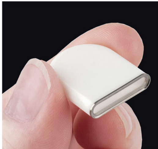
Fig. 4.25 Cylindrical brazen ceramic-Ti hermetic encapsulation, including battery, Bion. (Courtesy of Alfred Mann Foundation)
