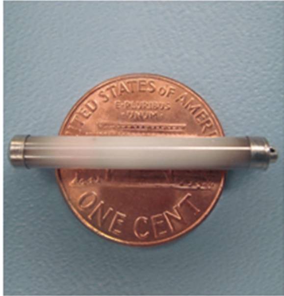
Fig. 4.24 Cylindrical brazed ceramic-Ti hermetic encapsulation, battery-less, Bion. (Courtesy of Alfred Mann Foundation)
