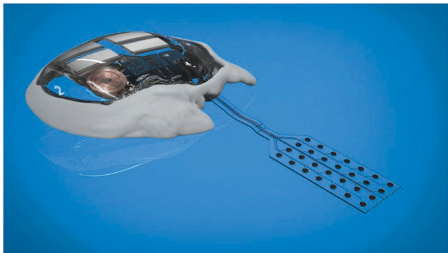
Fig. 5.4 Prototype of BCI integrated in a 3D laser-printed skull insert in PMMA. (This figure is reprinted with the permission of Longeviti Neuro Solutions LLC)
