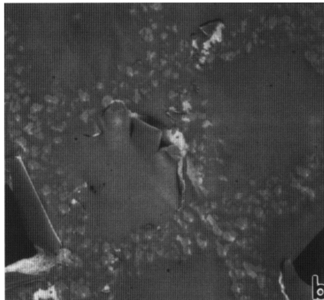
Example 1: Carbon foil on top of copper grid
