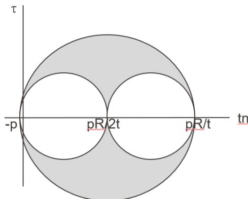
4 Use the von Mises criterion to show that failure could not be due to general yielding.
