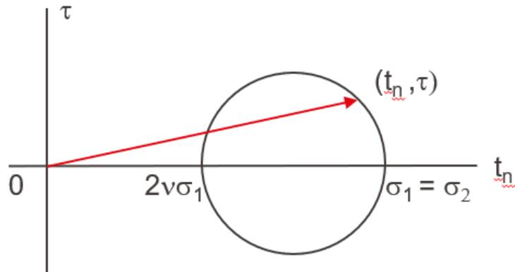
3. Deduce the first order estimate,  $r_y$ , of the plastic zone size under plain strain conditions. Calculate  $r_y$  assuming  $\nu = 1/3$  and compare this value with the estimate in plane stress conditions.
