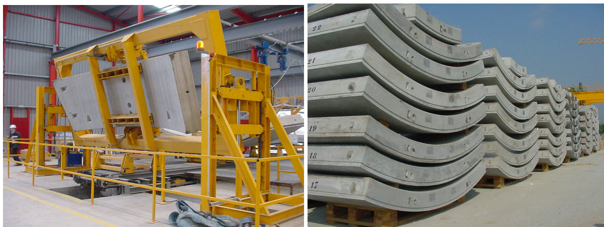
Fig. 7-18 Some of the transient load situations in which the segments are subjected to bending moments: (a) demoulding and (b) stacking at the yard
