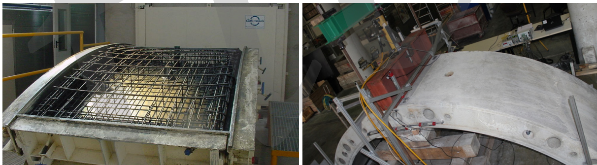
Fig. 7-17 Precast concrete segments: (a) Traditional reinforcement (Metro L9 of Barcelona) and (b) FRC full-scale bending test carried out at the UPC of Barcelona
