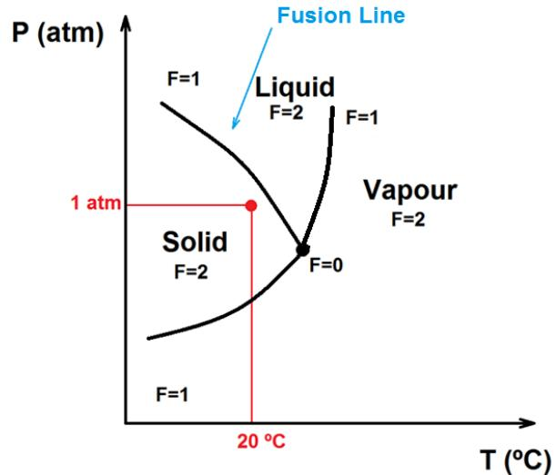
The slope of the vaporization line is unusually high.
