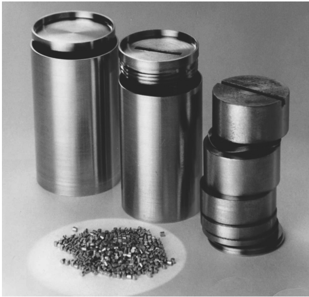
Figure 3. Cobalt pellets and source capsule with components.
