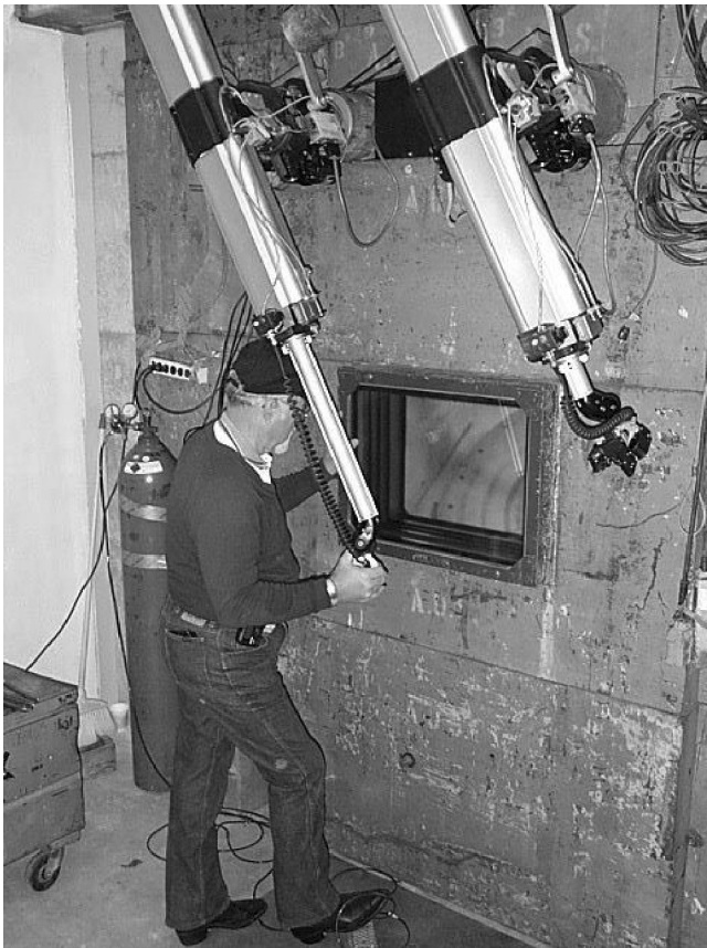
Figure 7. Loading cobalt-60 sources into Gamma Unit with remote manipulating arms.
