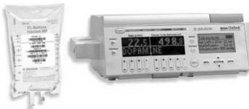
Figure 9. Outlook Safety Infusion System with DoseScan and DoseGuard by B|BRAUN technologies helping to ensure that the Right patient receives the Right medication in the Right dose from an authorized clinician at point of care.
