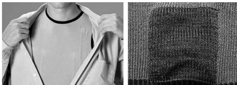
Figure 27. (a) The WEALTHY physiological monitoring vest with integrated sensors. (b) An early version of the fabric electrodes.
