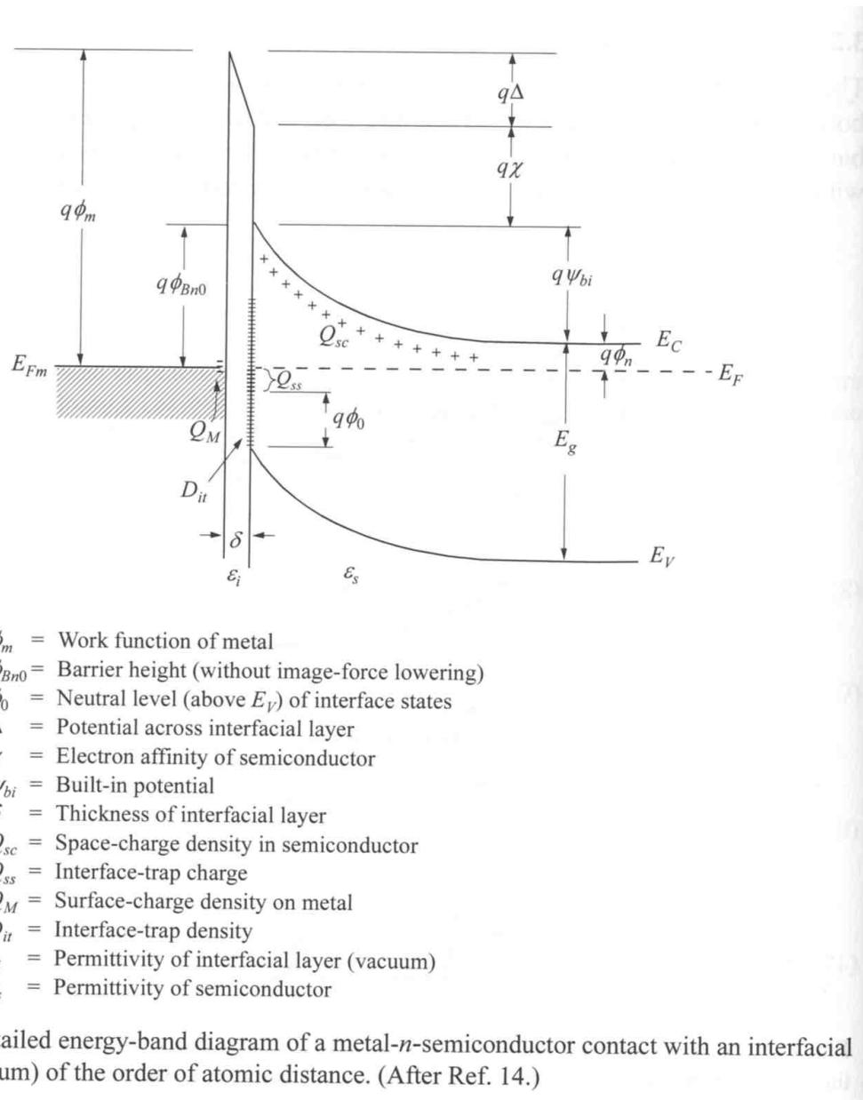
Figure 1: Schottky junction with interfacial layer.
