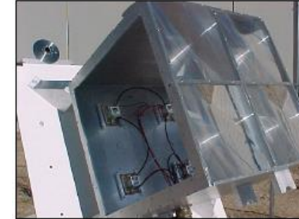
On-Sun testing at EMCORE Photovoltaics at 520 Suns
