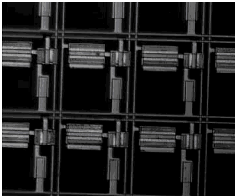
Figure 2: AMOLED pixel circuit.
