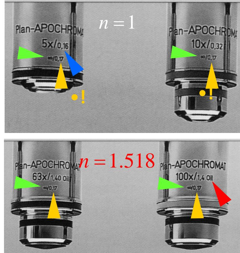
The NA defines how much light (signal) and how many diffraction orders (resolution) are captured by the objective.
