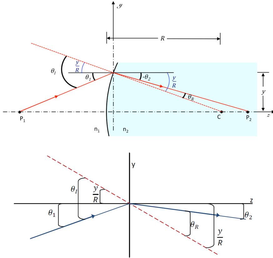
The red dashed line represents the radius of curvature, which is also normal to the surface. Snell's law relates the angle of incidence with the angle of refraction. We wish to derive a relationship between the angles of inc/ref with the angles formed by the z-axis (horizontal).
