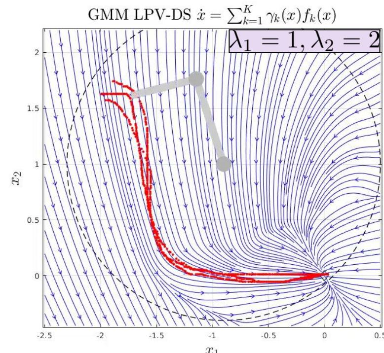
**Desired Behavior is determined by choice of damping eigenvalues.**
