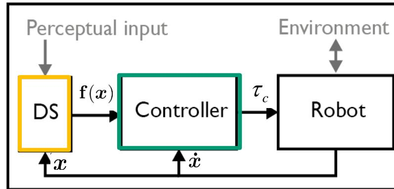
DS-based constant replanning of trajectory based on position feedback.
